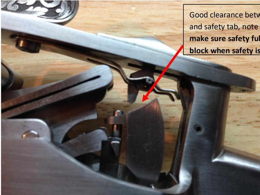
Good clearance between inertia block and safety tab, note trigger is cocked, **make sure safety fully retracts inertia block when safety is pulled back.**
