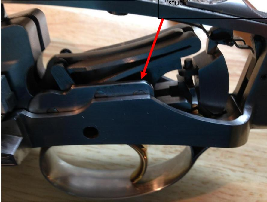
Tap down on trigger here if trigger gets "stuck"
