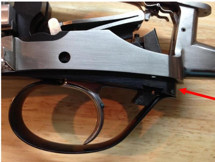
Typical distance trigger will not go in before fitting
